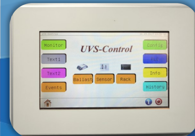
control unit with UV monitoring and USB ethernet interface
