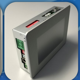
control unit with UV monitoring and USB ethernet interface
